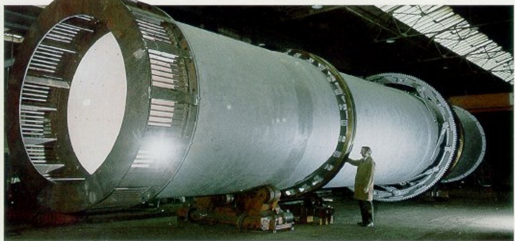
Rotary Air Cooler 3.4m dia x 17m
